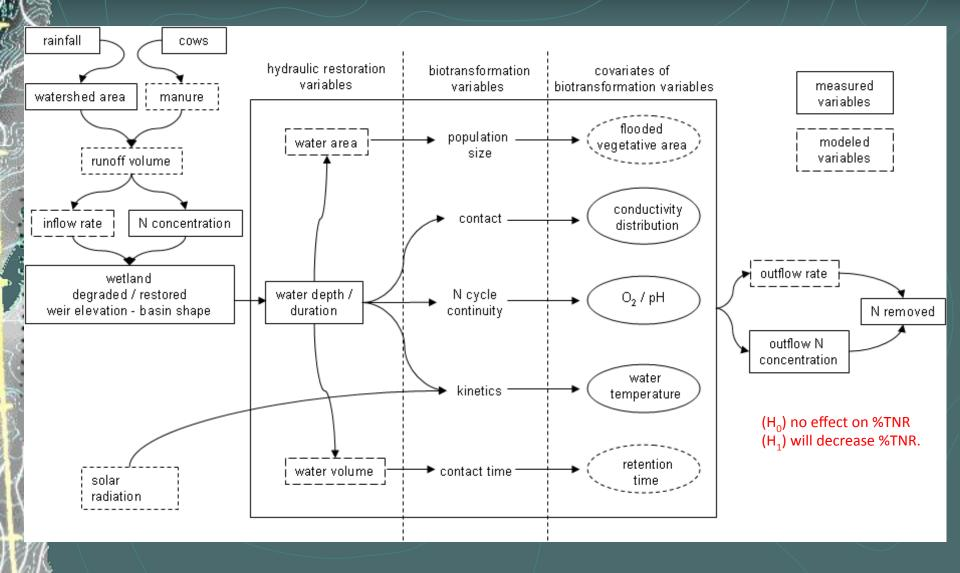
Hydraulic Restoration Variables: The flow diagram illustrates nitrogen polluted runoff interacting with wetland biotransformation variables and their as measurable covariates.
